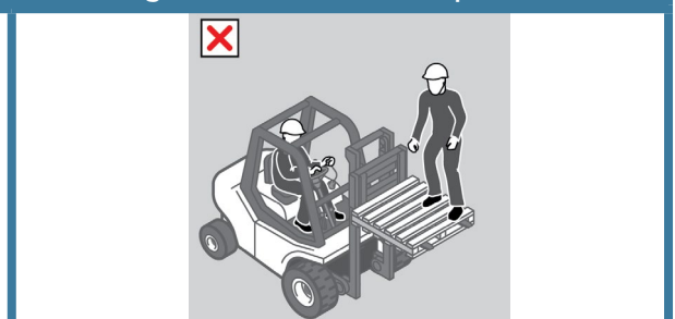
FIGURE 2 It is not safe to use a forklift as a work platform or to gain extra height by standing on the fork arms or a pallet
